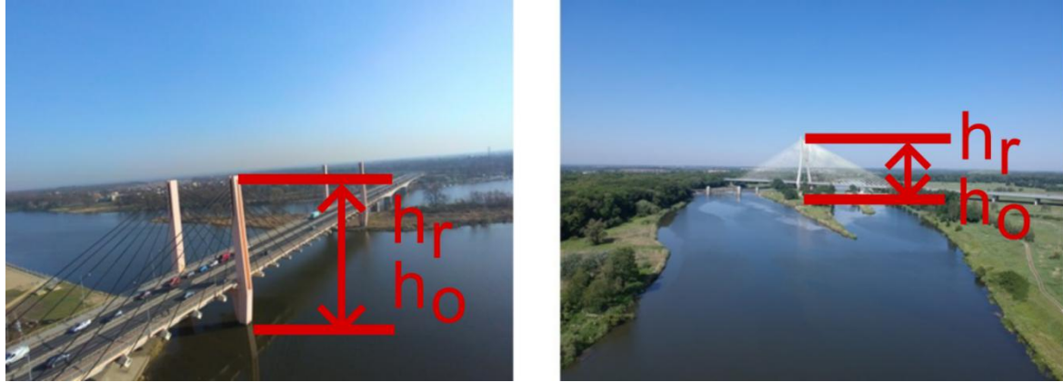
Fig. 2. Image (1): Yuneec Breeze 4K drone; h_r = 50\,000\text{mm} , h_o = 1212\text{px} , h_l = 3120\text{px} , real distance from the drone's camera is 98.3m (98310mm), distance estimated by proposed method is 128.7m (128713mm); image (2): image from DJI Spark drone; h_r = 125\,000\text{mm} , h_o = 736\text{px} , h_l = 2976\text{px} , real distance from the drone's camera is about 477m (477000mm), distance estimated by EstI method is 505.43m (505430mm)
