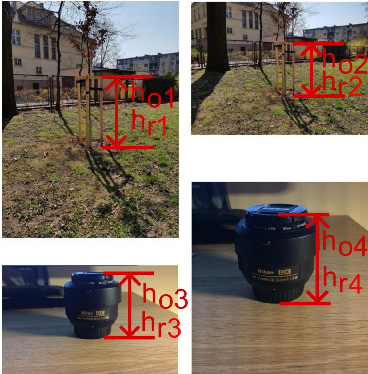
Fig. 3. The size of the object (in pixels) according to horizontal (landscape) and vertical (portrait) orientation. h_{r1} = 1500\text{mm} ; h_{r2} = 1500\text{mm} ; h_{r3} = 80\text{mm} ; h_{r4} = 90\text{mm} ; h_{o1} = 247\text{px} ; h_{o2} = 256\text{px} ; h_{o3} = 290\text{px} ; h_{o4} = 315\text{px}
