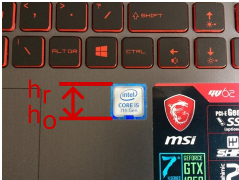
Fig. 1. Sample photograph used in experiment (Samsung S7). h_r = 17\text{mm} , h_o = 438\text{px} , h_r = 3024\text{px} , the real distance from the camera is 100mm, distance estimated with CPH / EstI method: 96mm / 117mm
