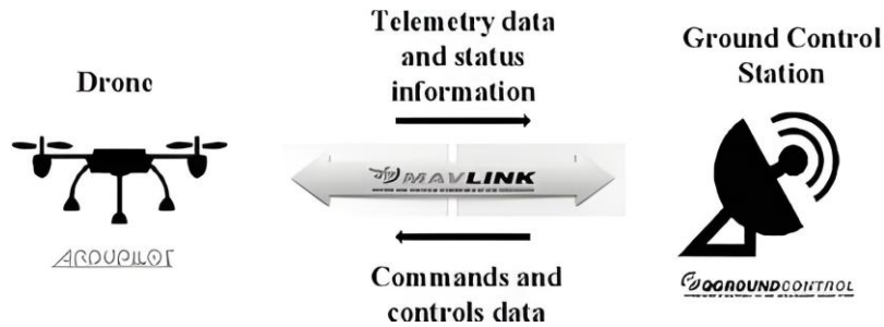
Fig. 2. Drone communication using MAVLink
