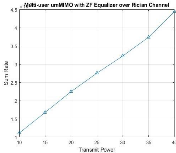
Fig. 10. Multi-user umMIMO with ZF equalizer over Rician Channel
