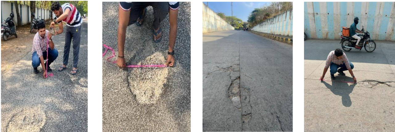
Fig. 1. Measurements of pavement distress along both flexible and rigid pavement
