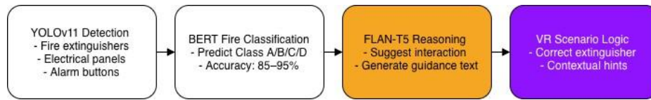
Fig.2. AI-driven scene intelligence pipeline illustrating object detection (YOLOv11), fire-class inference (BERT), and context-aware interaction guidance used during VR scenario execution
