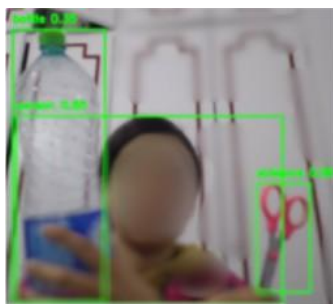
Fig.8. Output from live system: bottle detected upon voice command
