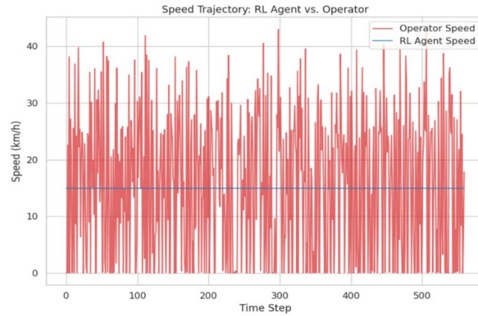
Fig.3. Time-series speed profiles of historical operator driving and the RL agent under identical operating conditions
