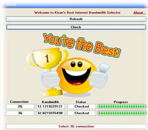
Fig 4: User interface of network selection algorithm based on available bandwidth estimation in heterogeneous environment of 2G and 3G network
