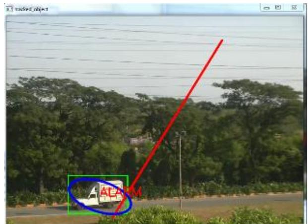
Fig.10 Vertical inclined trip wire (negative slope)
