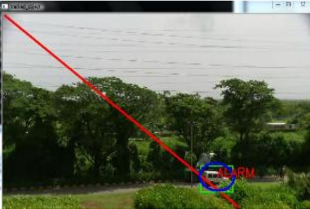
Fig.11 Vertical inclined trip wire (Positive slope)
