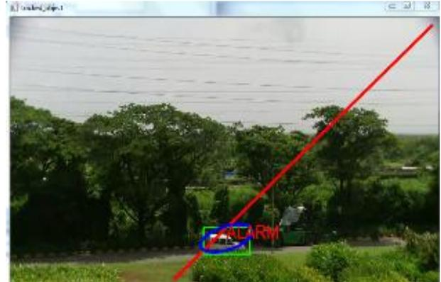
Fig.9 Vertical inclined trip wire (negative slope)
