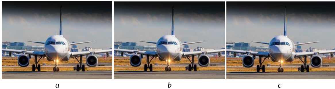
Fig. 7. Comparison of compressed images: a – original image (4948x3480x24b, 50447 Kbyte), b – compression by the wavelet method (JPEG-2000, 2971 Kbyte), c – compression by the proposed method (2700 Kbyte). The signal-to-noise ratio was: PSNR = 47.5 dB.
