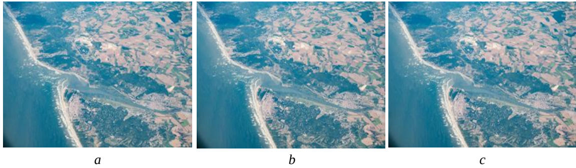
Fig. 6. Comparison of compressed images: a – original image (4288x2848x24b, 35779 Kb), b – compression by the wavelet method (JPEG-2000, 3578 Kbyte), c – compression by the proposed method (3276 Kbyte). The signal-to-noise ratio was: PSNR = 39 dB.
