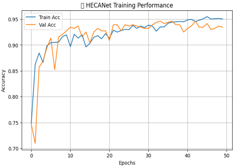
Fig. 3. Training and validation accuracy curves for the optimized HECANet model over epochs.
