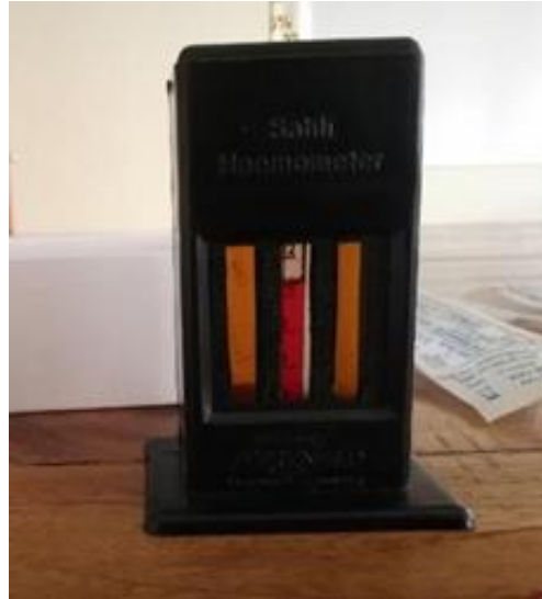
Fig. 2. Hb comparator box with brown glass on either side and a tube with acid hematin solution in the center. The color of the solution is matched with glass, and the concentration of Hb is read directly [33].
