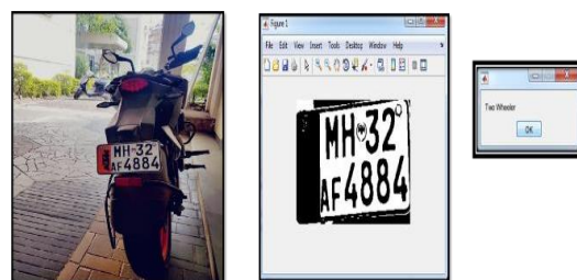
Fig.7. License plate and vehicle type detection (Two Wheeler).
