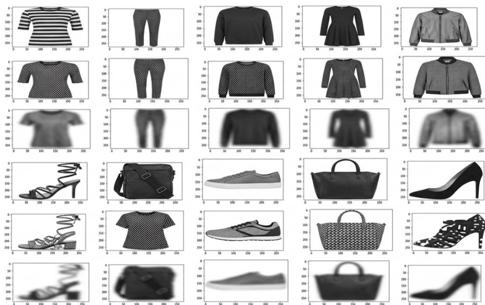
Fig. 5. Reconstructed images with learning rate 0.1 and hidden layer nodes 1000.
