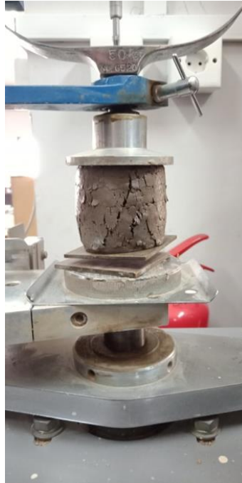
Fig. 3. Application of Load in UTM Machine, Geotechnical Engineering Laboratory, 2020
