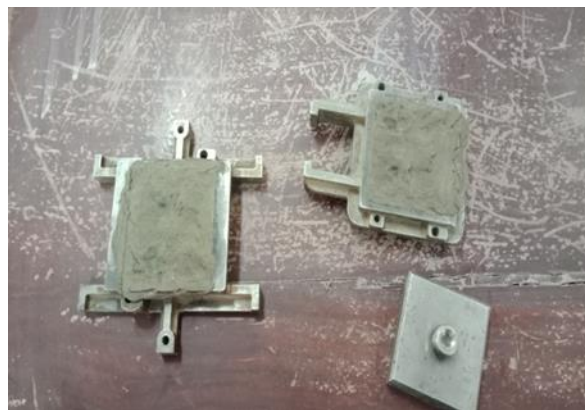
Fig. 4. Direct Shear Test Sheared Specimens, Geotechnical Engineering Laboratory, 2020
