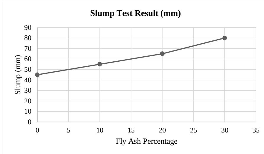
Fig. 1. Relationship between workability and fly ash replacement.
