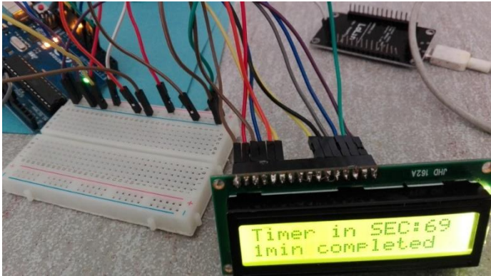
Fig. 6. Timer displaying in LCD 1 minute completed.
