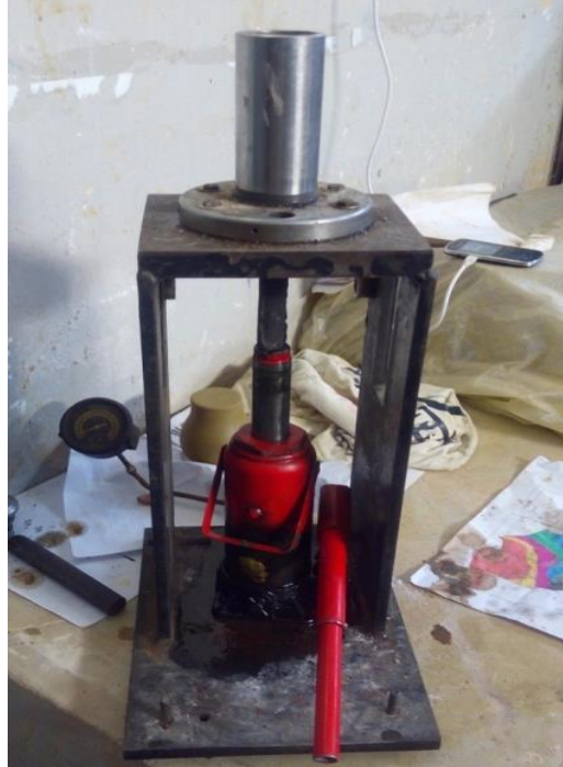
Fig.13. Press cast mould and hydraulic jack with pressure gauge
