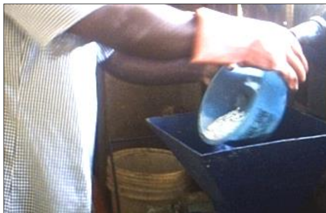
Fig.4. Pulverization of lump materials after sieving into fine particles
