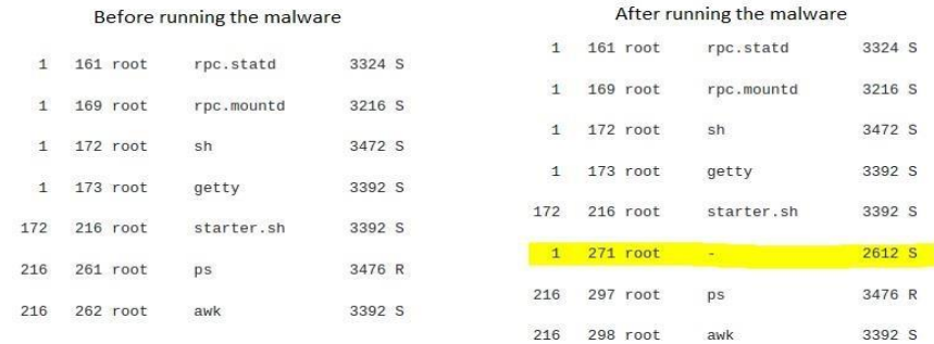
Fig.13. Process states before and after execution of malware
