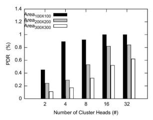
Fig. 2. Packet Delivery Ratio of 100 Nodes
