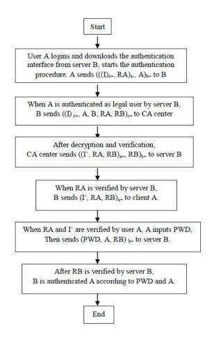
Fig 1. Authentication procedure of the ATTI login
