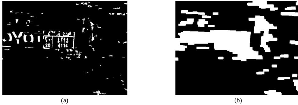
Fig.10. (a) Result of binarization & remove small regions, (b) Result of closing & dilation
