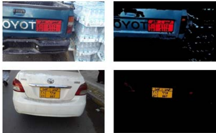
Fig.8. Samples of images after color filtering operation
