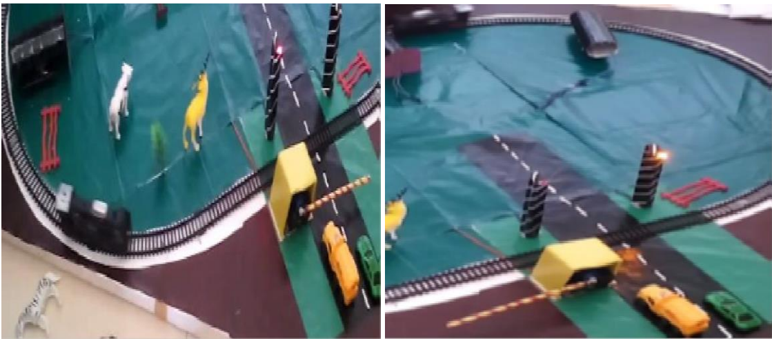
Fig.7. a) Train Approaching the Gate [Gate Closed and RED LED Was ON]. B) Train Leaving the Gate [Train Crossed the Gate, Gate Opened and Yellow LED Was ON]
