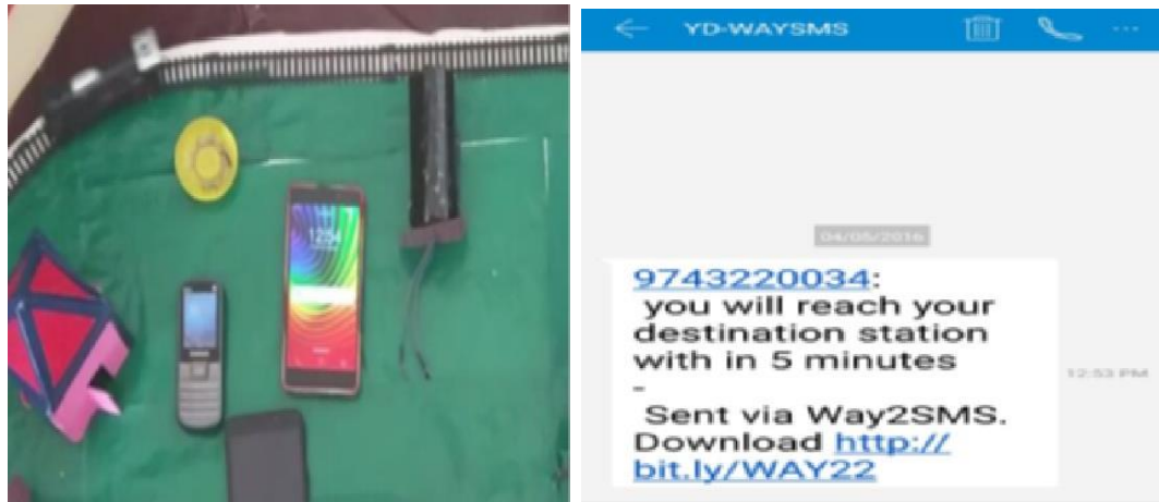
Fig.8. a) Train Approaching the Station [Two Registered Mobiles, Display on, Received the Alert Message and Another Mobile, Display Off, Is Not a Registered Mobile.]. b) Alert Message Format
