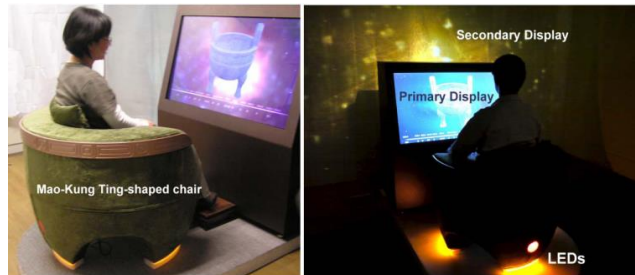
Figure 4: The installation has a primary display and a secondary display.
