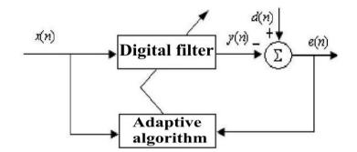
Fig. 5. Schematic diagram of adaptive filter algorithm
