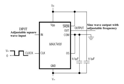
Fig. 3. Digital Filter Circuit
