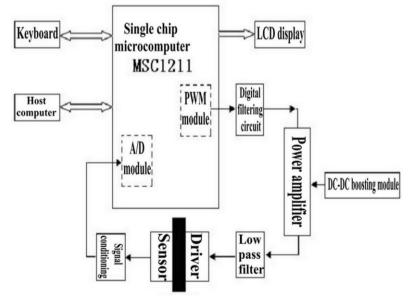
Fig. 1. Schematic diagram of active vibration control system
