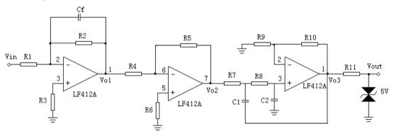
Fig. 2. Signal Conditioning Circuit
