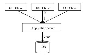
Fig 1. C/S two-tier architecture
