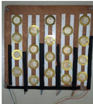
Fig. 3. Bottom View of the Piezoelectric Sensors and Spring Arrangement
