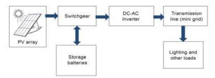
Fig. 1. A typical PV Microgrid [11]
