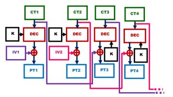
Figure. 11: Two-Way Interleaved CBC mode Decryption of PACTS
