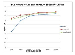
Figure. 4. Performance of ECB mode Encryption of PACTS
