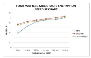
Figure. 16: Performance of 4-Way ICBC mode Encryption of PACTS
