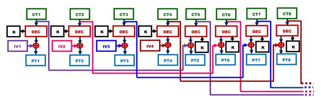
Figure. 15: Four-Way Interleaved CBC mode Decryption of PACTS
